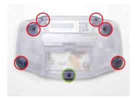
1) Remove highlighted screws with the Triwing and Philips screwdrivers. Pull shell apart.
