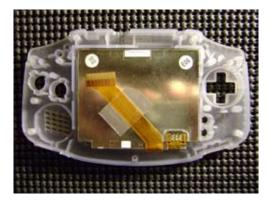
There protective film on the LCD. Do NOT remove it vet! Place new LCD into shell as shown.
