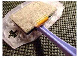
4) Remove LCD with a plastic pry tool or small flat head screwdriver, then pull away the sticky black border.
