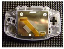
5) Place new LCD in the shell to test fit. Trim more plastic if needed until LCD sits flush.
