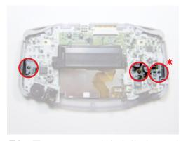
3) Remove highlighted Philips screws and remove the PCB.
